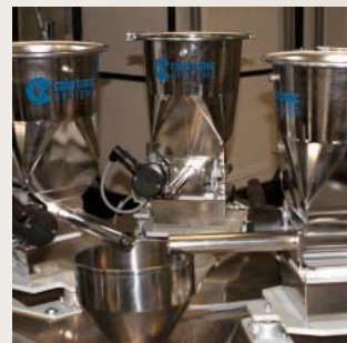
dosing equipment for twin-screw compounder
